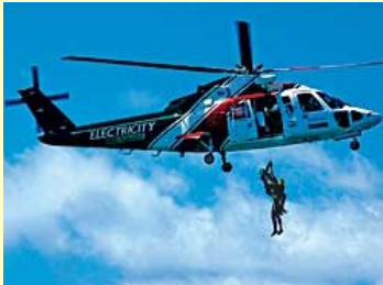
NEST's Sikorsky S-76A helicopter can carry two pilots, four medical attendants, and two patients on stretchers
